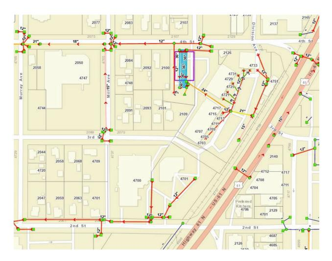
**Response 1:** Hydrologic boundary has been adjusted to reflect storm sewers in parking lot, southwest of Hwy 61 and 4th St interchange and adjusted parcels accordingly. Stormwater from this area flows west to vault under parking lot in VLAWMO. The legal boundary was reverted to its original boundary along US 61, following the hydrologic boundary.
